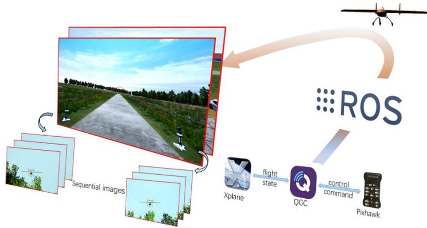
Fig. 2. Elaboration of Air2Land’s data generation scheme. Unlike simple picture synthesis, the real-world simulator is driven by flight control data generated by the hardware-in-the-loop system, and kinematic characteristics are passed from the controller to the drone model, then to the scene simulator, and finally naturally retained within the output sequence of images.
